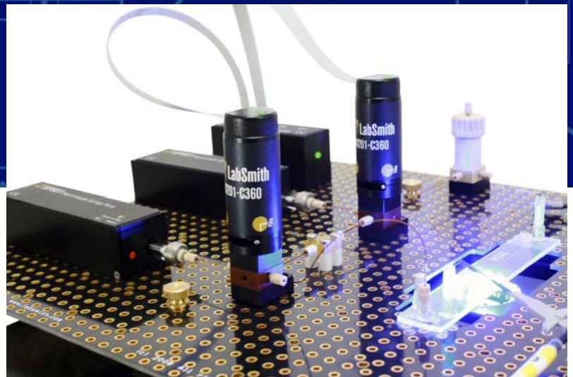
Figure 1. uProcess hardware, including: AV201 automated selector valves, SPS01 programmable syringe pumps, 4VM01 valve manifold, and IBB integrated breadboard. LabSmith's CapTite™ fluid routing components and a microfluidic chip complete this easy-to-use system for delivering micro- and nano-fluidic volumes.
