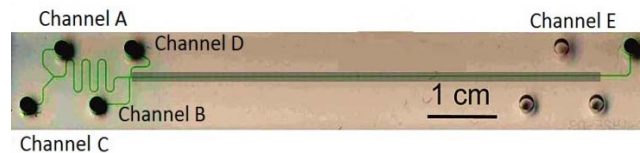
Figure 2. Gradient MEC Chip. Channels A and C contain the two elution buffers. Channel B is the Sample, Channel D is Sample Waste, Channel E is Buffer Waste.
